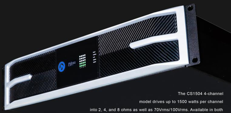
Network Connect (CS1504) and Dante Connect (CS1504D) versions, the D-model includes both 96 kHz-capable Dante and AES67 connectivity options. These units also utilize our most advanced DSP with 96kHz linear phase FIR crossover filters, acoustically transparent look ahead RMS and peak limiters, plus 32-bit floating-point DSP with built-in sample rate converters. The CS1504 sets the standard in pro audio amplifier performance, connectivity, and ease of deployment for large installations.
